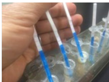
Fig.2 RoundupReady soybean screening test kit (Lateral Flow)
