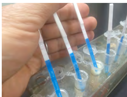
Fig.2 RoundupReady soybean screening test kit (Lateral Flow)
